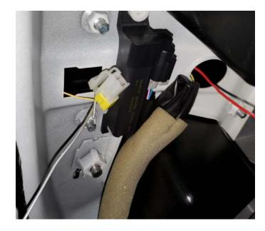
**20.** Install ground on stud as shown:
