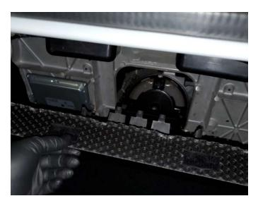
**11.** Remove the styrofoam section at the forward section of the trunk and cut it as follows:
