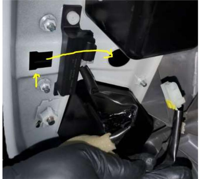
**18.** Open the wire loom to expose the yellow power wire and utilize the included connector to connect the red and yellow wires as shown):
