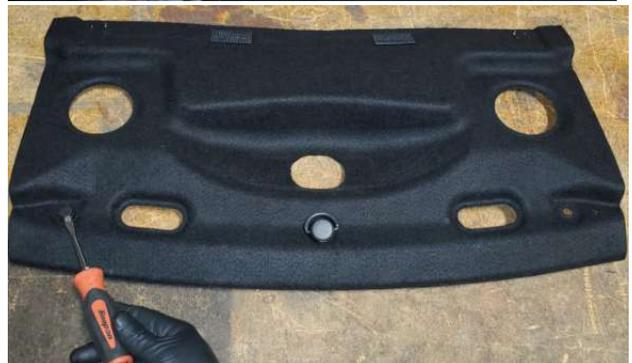
**10.** Pull the side clips and remove the panel with the Velcro:
