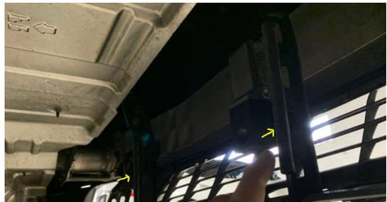
4. Install the AAM Competition muffler section. Slide the four hanger rods into the factory rubber hanger mounts:
