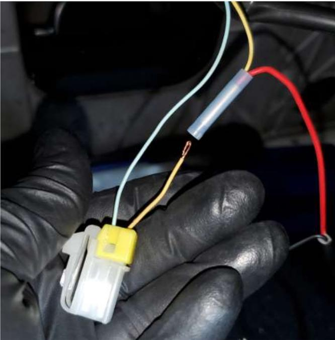
**19.** Use a fish wire (such as a coat hanger) to pull the wire back through the round hole to the rectangular style hole:
