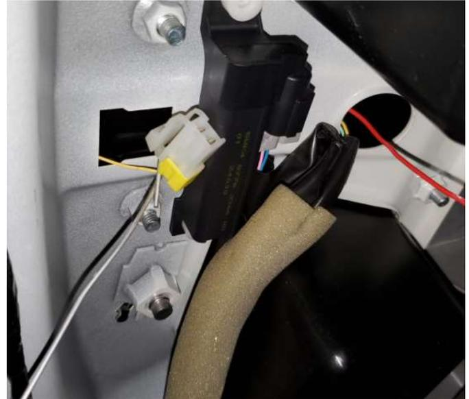
**20.** Install ground on stud as shown:
