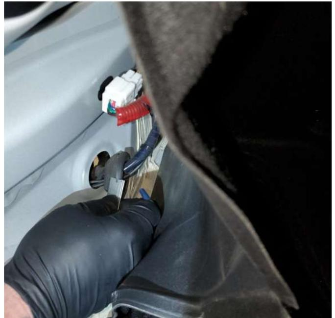
**14.** Connect the antenna, vacuum line, and power cable to the vacuum generator as shown:
