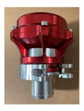
**12.** Install the Tial BOV on the AAMC BOV couplers. Adjust the positioning as necessary to allow enough space for the BOV. Move and adjust the A/C hard line as shown below to allow room for the Tial BOV. Do not tighten and clamps yet!
