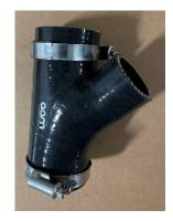
**10.** Install the new AAMC BOV couplers as shown below. Orient the BOV port of the coupler towards the headlights of each respective side. Grab the supplied worm gear clamps and place them on the open port as shown, do not tighten any worm gear clamps to allow adjustability of the blow off valve final location.
