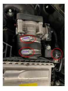
**5.** Use a 7mm socket to loosen the 4 worm gear clamps on the passenger and driver side intercooler couplers, use ratchet extensions as needed.
