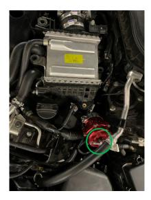
**14.** Carefully remove the OEM PCV Hose behind the intake manifold and driver side throttle body as shown below. This hose connects a hard line to the plastic PCV nipple on the intake manifold.
