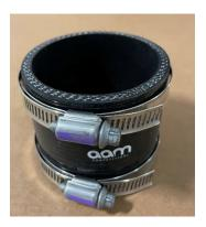
**8.** Install the AAMC throttle body couplers, ensuring the clamps are loose to allow movement of the intercoolers when installing the new AAMC intercooler BOV couplers.
