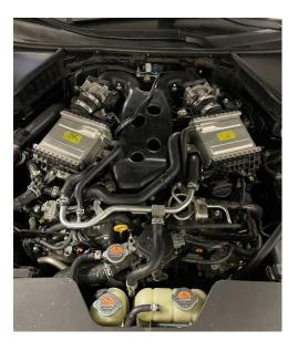
3. Remove the 8 x 12mm bolts holding the passenger and driver side intercoolers.
