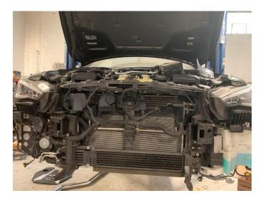
15. Remove the bolts from the oil cooler, then use zip ties to keep it out of the way.
