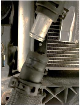
18. Disconnect the return hose from the next T-fitting, using pliers to slide the clamp up the hose. Make sure the T-fitting does not come out of the other hose. The clamp will be reused.
