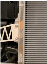
**21.** Attach the rubber grommet to the left bracket and heat exchanger.
