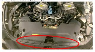
**8.** There are two hidden bolts where the trim meets the bumper on both sides. Remove them and the brackets they hold in place. Carefully slide the bumper off of the vehicle.
