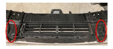
**14.** Prop up the crash beam so that it will not fall, then remove the last bolts from each side. Store in a safe place.
