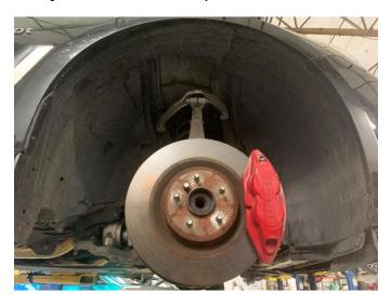
**4.** Remove the wheel well liners on each side by disconnecting all push clips.
