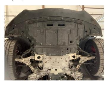
**3.** Remove front wheels from the vehicle using the proper wheel lug removal tool and socket for your model.
