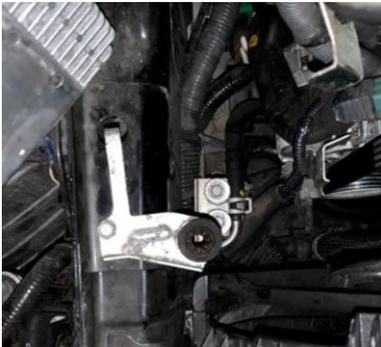
7. Disconnect the rear half of the air box from the metal clip underneath by using two screwdrivers to pry out the clamp, then lift the air box up. The image below shows the clamp already disconnected.
