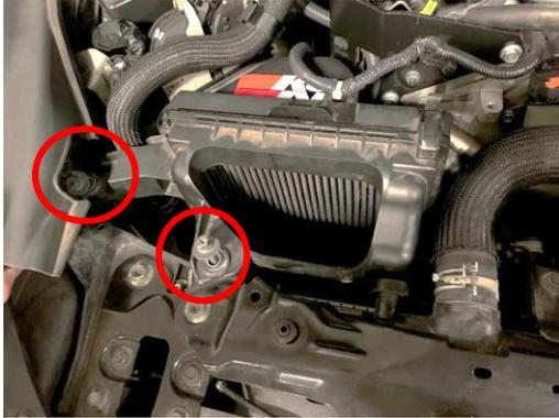
4. Release the front of the air box from the car by pulling upwards to remove it from the rubber grommet underneath.
