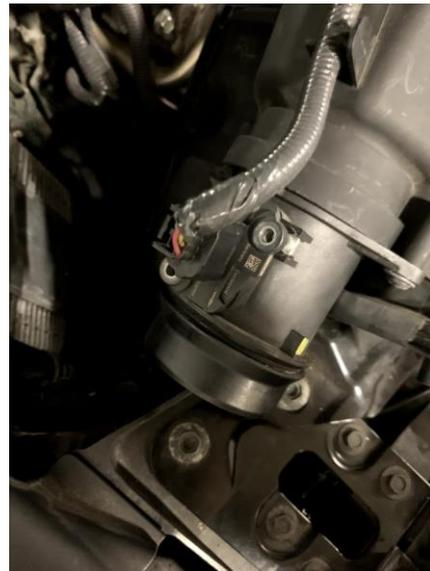
9. Remove the OEM turbo hose by unscrewing the pipe clamp on the bottom of the hose with an 8mm socket or flathead screwdriver. Then, use pliers to remove the PCV hose from the upper port.
