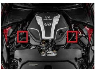
Red Boxes are where you should be able to fit socket with extension down to the top nuts.
