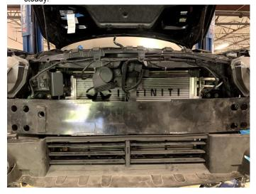
**14.** Prop up the crash beam so that it will not fall, then remove the last bolts from each side. Store bolts and beam in a safe place. Tip: Have a buddy hold this piece when removing it. It's quite a bit easier!
