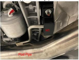
4. Install the AAM Competition muffler section. Bolt the 4 hanger bracket mounts back to their respective stud locations on the car. Add the supplied spacers between the studs and the hanger bracket mounts to ensure proper fitment of the exhaust tips. Use an under hoist support stand to help hold the exhaust.
