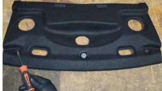
**10.** Pull the side clips and remove the panel with the Velcro:
