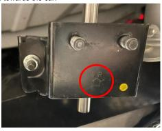
3. Install the AAM Competition Post Pipe as shown below. Mount the hanger bracket back to its location marked H1 in the pictures above. Use the supplied bolts, nuts and washers (two bolts and nuts per side, four washers per side) to attach the post pipe to the GT-R's mid-pipe. Leave this slightly loose for now.
