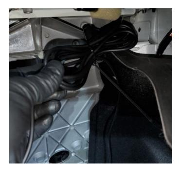
**22.** Run vacuum line as shown, through the modified grommet and underneath the GT-R to the exhaust actuator:
