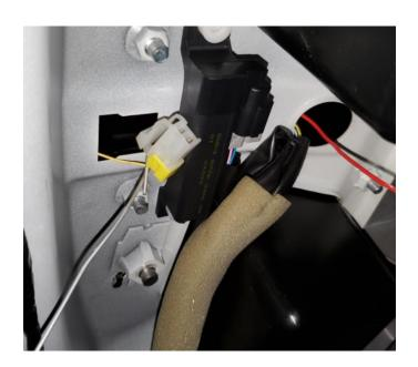
**20.** Install ground on stud as shown:
