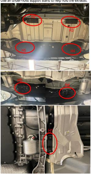
2. Remove the hanger bracket mounts from the stock exhaust hangers. Re-install the hanger bracket mounts on the new AAM exhaust. Ensure the hangers bracket mounts are installed on the correct hanger and they are oriented properly. (Each hanger bracket mount has an arrow indicating the orientation to be installed towards the car.
