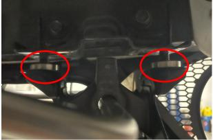
**5.** Use the supplied V-Band clamp to connect the post pipe to the muffler section. Do not fully tighten yet.
