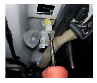
**17.** Pull and remove harness through circular hole, to allow you to connect the power supply as shown:
