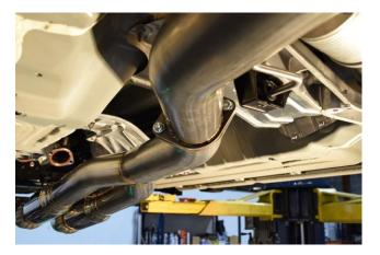
14. Bolt the front flanges of the midpipe to the bottom of the downpipes using the supplied hardware.
