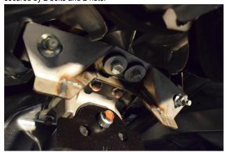
**6.** Disconnect and remove the front drive shaft. There are 4 hex bolts securing each end of the shaft.
