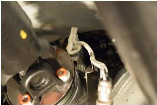
**8.** Disconnect the upper o2 sensor harness clips from each of the OEM downpipes. The upper o2 sensor clips are accessible from the top of the engine bay.
