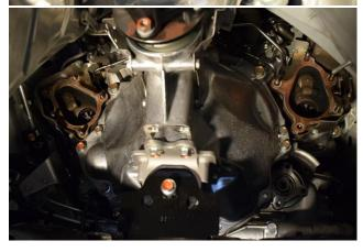
10. Carefully remove the o2 sensors from your original downpipes and install them into the AAM Competition GT-R Downpipes. Be sure to note the location of each o2 sensor in the OEM downpipes, as they will need to be installed in the same location on the new downpipes.
