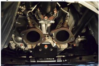
**5.** Remove the mounting bracket beneath the OEM downpipes, secured by 2 bolts and 2 nuts.
