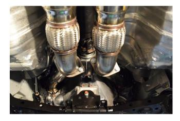
**7.** Once the AAM Competition GT-R Midpipe is properly positioned, fully tighten all hardware.
