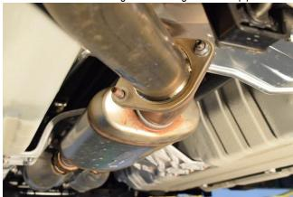
**4.** Remove the midpipe by uninstalling the 4 bolts securing the front flanges to the bottom of the downpipes.
