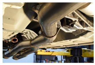
**6.** Bolt the front flanges of the AAM Competition GT-R Midpipe to the bottom of the downpipes. (See image at top right of page)
