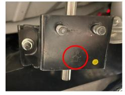
3. Install the AAM Competition Post Pipe as shown below. Mount the hanger bracket back to its location marked H1 in the pictures above. Use the supplied bolts, nuts and washers (two bolts and nuts per side, four washers per side) to attach the post pipe to the GT-R's mid-pipe. Leave this slightly loose for now.
