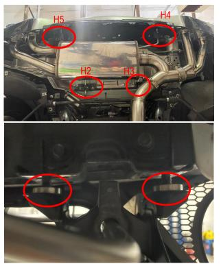
**5.** Use the supplied V-Band clamp to connect the post pipe to the muffler section. Do not fully tighten yet.
