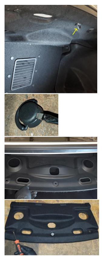
**10.** Pull the side clips and remove the panel with the Velcro:
