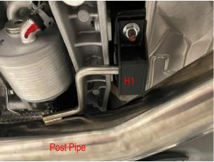
4. Install the AAM Competition muffler section. Bolt the 4 hanger bracket mounts back to their respective stud locations on the car. Add the supplied spacers between the studs and the hanger bracket mounts to ensure proper fitment of the exhaust tips. Use an under hoist support stand to help hold the exhaust.
