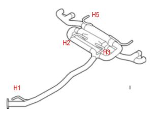
Use an under-hoist support stand to help hold the exhaust.
