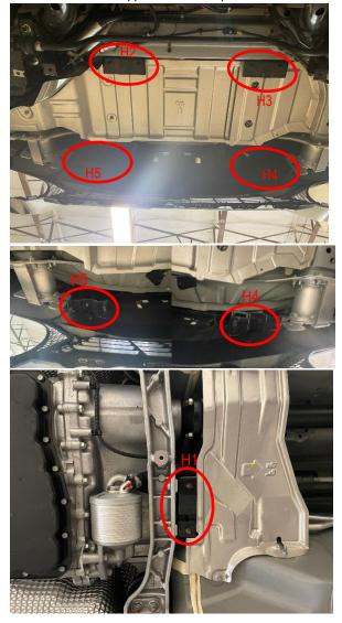
2. Remove the hanger bracket mounts from the stock exhaust hangers. Re-install the hanger bracket mounts on the new AAM exhaust. Ensure the hangers bracket mounts are installed on the correct hanger and they are oriented properly. (Each hanger bracket mount has an arrow indicating the orientation to be installed towards the car.
