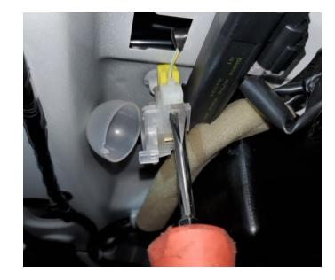
**17.** Pull and remove harness through circular hole, to allow you to connect the power supply as shown:
