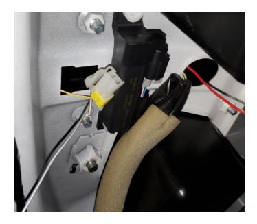
**20.** Install ground on stud as shown:
