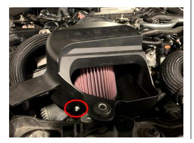
**22.** Secure the Intake Box using the 10mm bolts from the OEM air box.
