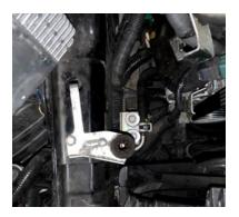
Disconnect the rear half of the air box from the metal clip underneath by using two screwdrivers to pry out the clamp, then lift the air box up. The image below shows the clamp already disconnected.
