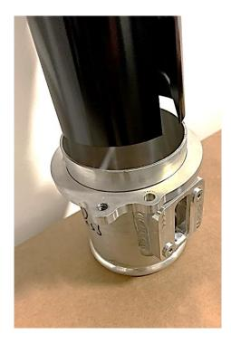
**19.** Secure the air filter to the AAM Competition MAF Housing through the bottom port with a flathead screwdriver.
