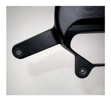
**21.** Place the top half of the AAM Competition Intake Box on top, and install the two side screws with a 3mm hex head wrench. One screw is in the front, one screw is in the back.
