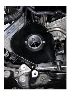
**18.** Insert the AAM Competition MAF Insert into the MAF Housing, carefully sliding it so that the MAF sensor rests in the slot. The orientation is shown in the image below, outside of the car for clarity:
