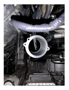
**17.** Screw the lower half of the AAM Competition Intake Box onto the MAF Housing.
