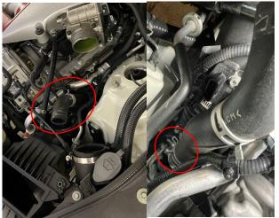
**8.** Grab the AAM Competition upper intercooler pipes and install the provided couplers in the orientation shown below:
