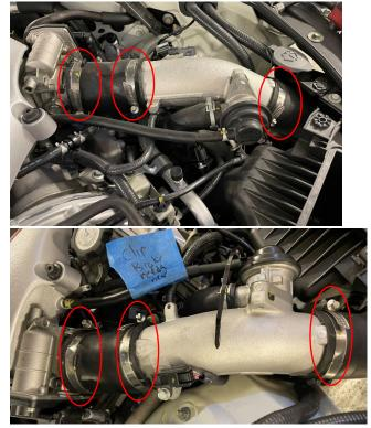
Once all clamps have been loosened, remove both upper intercooler pipes along with the throttle body couplers attached to both ends of the pipe.
