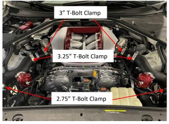
Connect the vacuum lines to the BOVs. Tighten all clamps and the installation is done!
