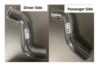
10. Install the upper intercooler pipes, use the correct sized clamp on each end as shown below. Install the Tial BOV on the flange as shown. Connect the recirculation tube to the BOV using the supplied worm drive clamps.
