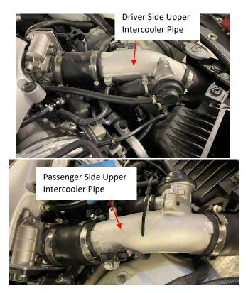
**4.** Disconnect the vacuum line and hose going into the stock blowoff valves on the upper intercooler pipes. Use pliers to remove the clamps.
